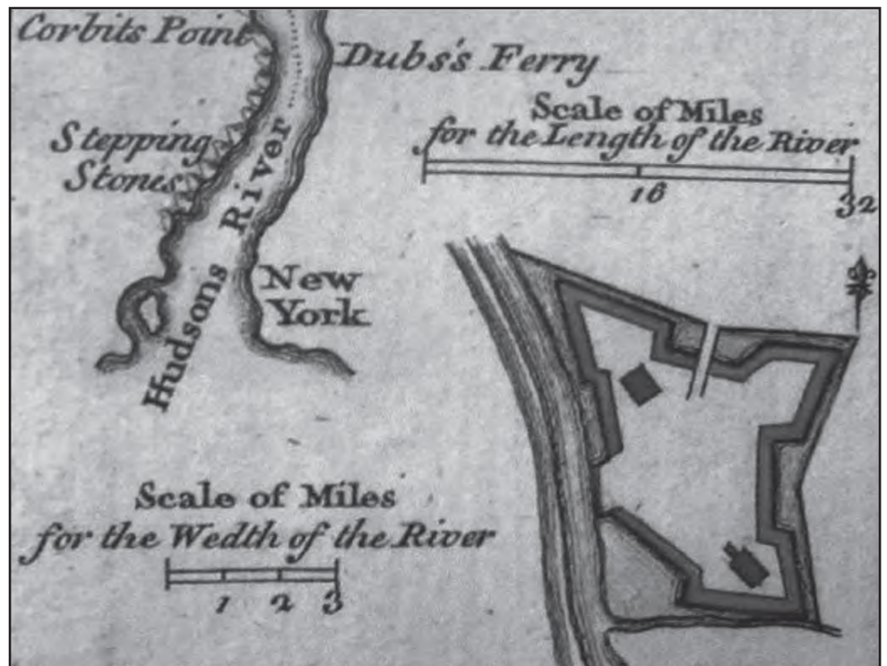
This detail from Blodget’s Hudson River map shows that he used different north-south and east-west scales.
