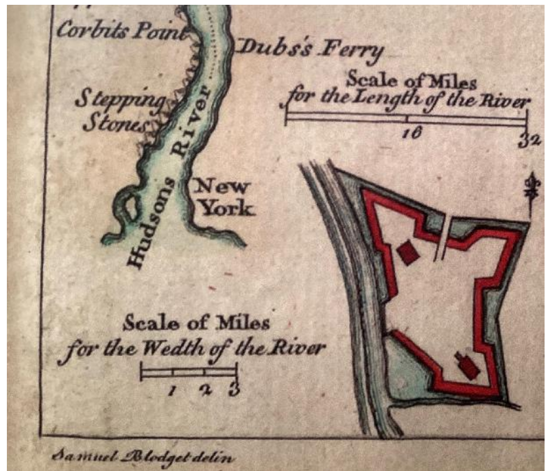
Figure 5. Detail from the Hudson River panel of Blodget's drawing showing differing east-west and north-south scale bars.
