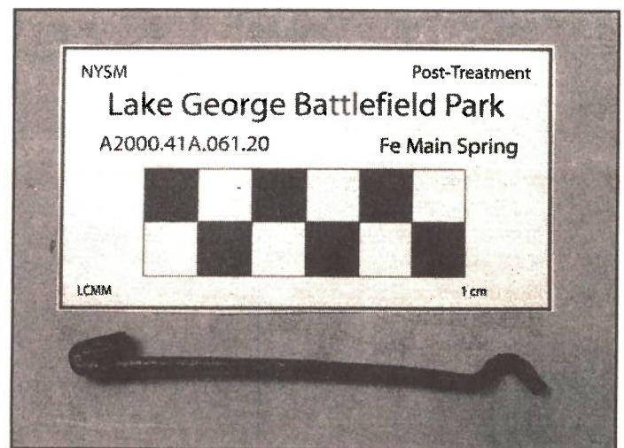
(Figure 3) Musket Lock Main Spring. (courtesy of the Conservation Laboratory, Lake Champlain Maritime Museum)
